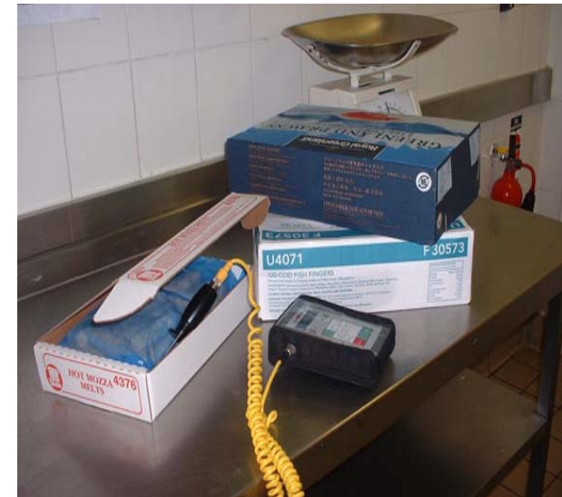
Thermometer probing of food between packs
